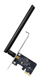
The Archer T2E receives Wi-Fi signals on two separate bands for all your online needs. Choose the 2.4 GHz band for browsing, email and social media, or switch to 5 GHz band for gaming and streaming. The Archer T2E can work with MU-MIMO routers, which provide simultaneous data streams, boosting throughput and efficiency.
